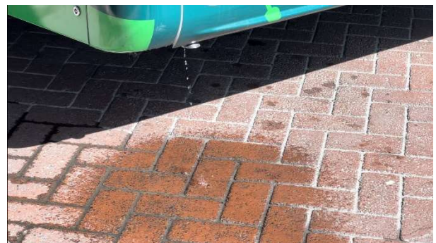
The exhaust on 1788, emitting steam and hot water, not the traditional greenhouse gas emissions! – 5/9/23 - Matthew Schoepf
